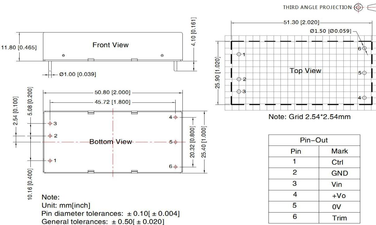
Horizontal Package Dimensions (with heat sink)
