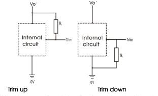
TRIM resistor connection (dashed line shows internal resistor network)
