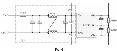
Notes: For EMC tests we use Part (1) in Fig. 4 for immunity and emissions test.
