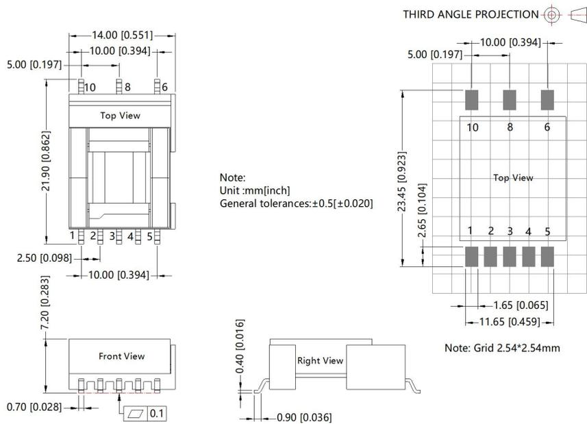
TTL503-15B12T Dimensions and Recommended Layout
