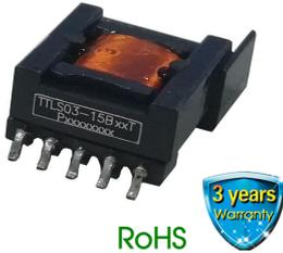
TTL503-15BxxT transformer series feature with 3000VAC primary to secondary isolation, an operating ambient temperature range of -40°C to +110°C. It can be used with our control IC SCM1702ASA to achieve flyback power supply design with wide input voltage range and various protection functions and superior EMI performance.
