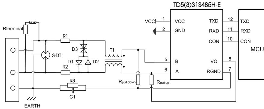
Fig. 2: Port protection circuit for harsh environments
