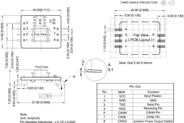
Pin diameter tolerances:  $\pm 0.10[\pm 0.004]$ General tolerances:  $\pm 1.0[\pm 0.039]$
