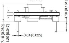
Pin diameter tolerances:  $\pm 0.10[\pm 0.004]$ General tolerances:  $\pm 1.0[\pm 0.039]$
