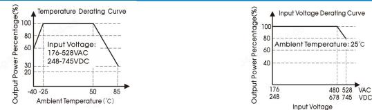
Note: 1) With an AC input between 480-528VAC and a DC input between 678-745VDC, the output power must be derated as per temperature derating curves; 2) This product is suitable for applications using natural air cooling; for applications in closed environment please consult Mornsun FAE.
