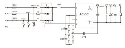
Fig. (2): Recommended circuit for applications which require 4KV differential-mode surge standard (half-wave rectification)
