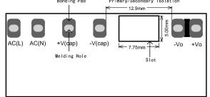
Note: There is a slot(non-metallic hole) between pin 4/5; For details, please refer to the recommended dimensions or pad.
