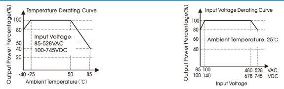
Note: 1) With an AC input between 85 -100V/480-528VAC and a DC input between 100 - 140V/678-745VDC, the output power must be derated as per temperature derating curves;
