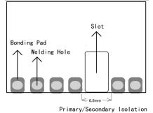
Note: There is a slot(non-metallic hole) between pin 4/5, For details, please refer to the recommended dimensions or pad.
