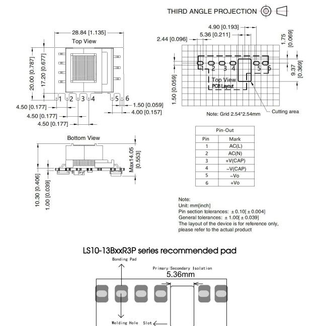
Note: There is a slot(non-metallic hole) between pin 4/5, For details, please refer to the recommended dimensions or pad.
