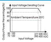
Note: ① With an AC input between 85-100VAC/277-305VAC and a DC input between 70-120VDC/390-430VDC, the output power must be derated as per temperature derating curves;
