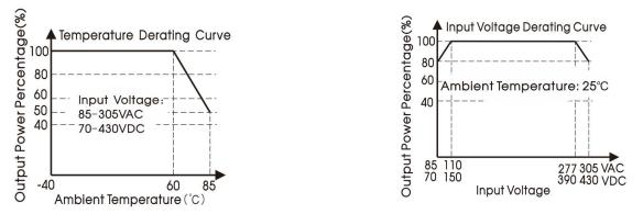
Note: 1) With an AC input between 85 -110VAC/277- 305VAC and a DC input between 70 - 150VDC/390 - 430VDC, the output power must be derated as per temperature derating curves;
