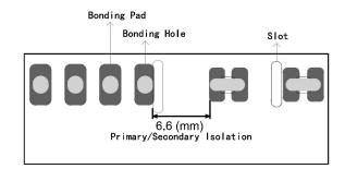
Note: There is a slot(non-metallic hole) between pin 4, which the side pad were being cut off. For details, please refer to the recommended dimensions or pad.
