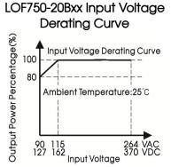
Note: With an AC input voltage between 90 - 115VAC and a DC input between 127 - 162VDC the output power must be derated as per the temperature derating curves.
