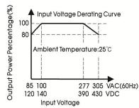
Note: 1. With an AC input voltage between 85 -100VAC and a DC input between 120-140VDC the output power must be derated as per the temperature derating curves;
