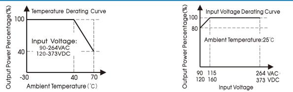
Note: 1. With an input voltage between 90 -115VAC and a DC input between 120-160VDC the output power must be derated as per the temperature derating curves;
