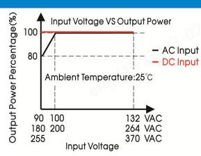
Note: 1. With an AC input voltage between 90 - 100VAC/180 - 200VAC and a DC input 255 - 370VDC must be derated as per the temperature derating curves; 2. This product is suitable for applications using forced air cooling; for applications in closed environment please consult Mornsun FAE.
