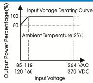
Note: 1. With an AC input voltage between 85 - 115VAC and a DC input between 120 - 160VDC the output power must be derated as per the temperature derating curves;
