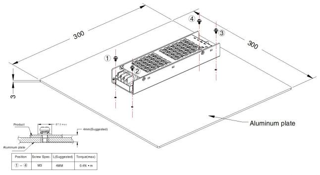
1. In order to meet the "Derating Curve", the product testing must be installed onto an aluminum plate. The size of the suggested aluminum plate is shown as above. And for optimizing thermal performance, it is necessary to apply thermal grease on the bottom of the product.
