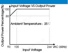
Note: 1. With an input voltage between 90-100VAC the output power must be derated as per the temperature derating curves;
