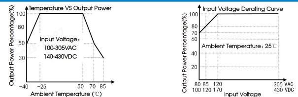
Note: 1) With an AC input between 80-120VAC and a DC input between 100-170VDC, in addition to the voltage drop, temperature derating is also required. If it is used in a low temperature environment, please consult Mornsun FAE.
