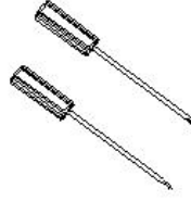
Phillips screwdriver Slotted screwdriver Diameter : 3mm
