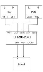
Note: 1. Please add AC-DC module at front of LIHR40-20-H (Mornsun LI, LIF, LIMF, LIHF120/240/480/960 series products are recommended); 2. When the output is short circuited, the pre-stage AC-DC module short circuit protection will be triggered;
