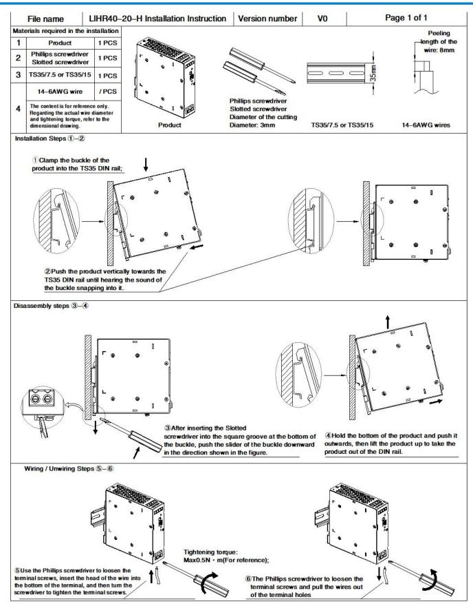
Note: Keep the following installation clearances: 20mm on top, 20mm on the bottom, 5mm on the left and right sides are recommended when the device is loaded permanently with more than 50% of the rated power. Increase this clearance to 15mm in case the adjacent device is a heat source (e.g. another power supply).
