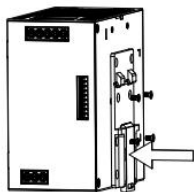
① Mounting the universal DIN rail power supply. (Forward Installation. Label is needed to be removed)
