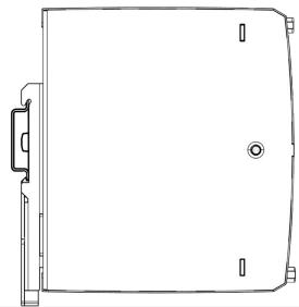
Note: Keep the following installation clearances: 20mm on top, 20mm on the bottom, 5mm on the left and right sides are recommended when the device loaded permanently with more than 50% of the rated power. Increase this clearance to 15mm in case the adjacent device is a heat source (e.g. another power supply).
