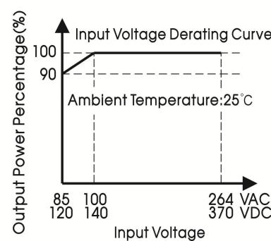
Note: 1. With an AC input voltage between 85 -100VAC and a DC input between 120-140VDC the output power must be derated as per the temperature derating curves;
