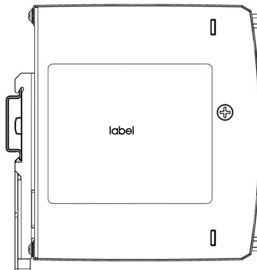
Notice: Keep the following installation clearances: 20mm on top, 20mm on the bottom, 5mm on the left and right sides are recommended when the device is loaded permanently with more than 50% of the rated power. Increase this clearance to 15mm in case the adjacent device is a heat source (e.g. another power supply).
