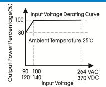
Note: 1. With an AC input voltage between 90 -100VAC and a DC input between 120-140VDC the output power must be derated as per the temperature derating curves;
