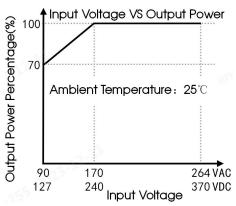
Note: 1. With an AC input voltage between 90 -170VAC and a DC input between 127-240VDC the output power must be derated as per the temperature derating curves;
