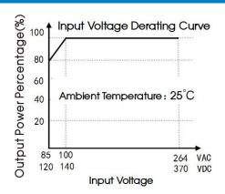
Note: ① With an AC input between 85-100VAC and a DC input between 120-140VDC, the output power must be derated as per temperature derating curves; ② This product is suitable for applications using natural air cooling; for applications in closed environment please consult Mornsun FAE.
