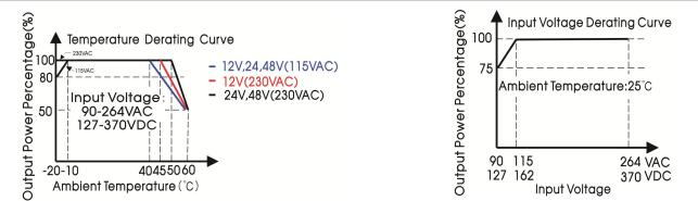
Note: 1.With an AC input voltage between 90-115VAC and a DC input between 127-162VDC the output power must be derated as per the temperature derating curves;
