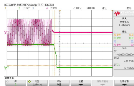
Vin=230VAC Full load shutdown (46ms)
