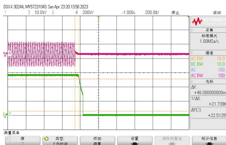
Vin=115VAC Full load shutdown (46ms)
