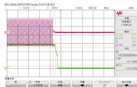
Vin=230VAC Full load shutdown (46ms)
