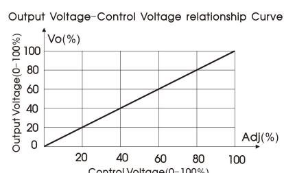
Fig.3 The relationship curve of output voltage and control voltage
