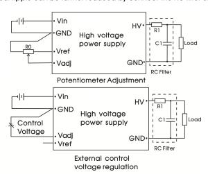
Fig. 2 External adjustment method of output voltage
