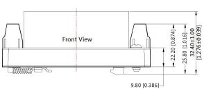
Note: Unit: mm[inch] Wire range: 24-12 AWG Tightening torque: Max 0.4 N·m Installed on DIN RAIL TS35 General tolerances: ±0.50[±0.020]
