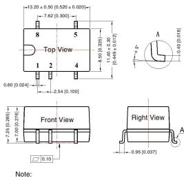
Unit: mm[inch] Pin section tolerances:  $\pm 0.10[\pm 0.004]$ General tolerances:  $\pm 0.25[\pm 0.010]$
