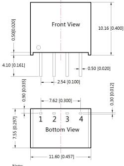
Note: Unit :mm[inch] Pin section tolerances:±0.10[±0.004] General tolerances:±0.25[±0.010]
