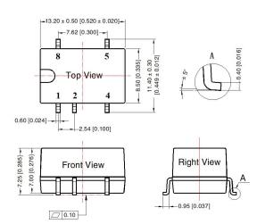
Note: Unit: mm[inch] Pin section tolerances:  $\pm 0.10[\pm 0.004]$ General tolerances:  $\pm 0.25[\pm 0.010]$
