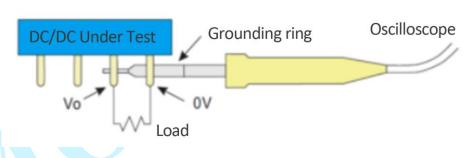
Diagram 2-4 Contact measuring method with oscilloscope
