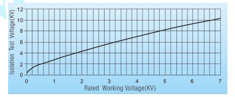
Diagram 2-8 Relationship between Isolation Test Voltage and Rated Working Voltage
