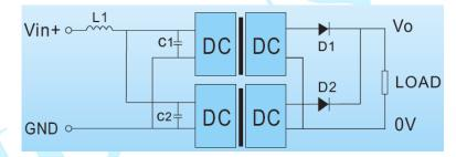
Diagram 3-3 Method 1 of DC/DC Converters connected in parallel
