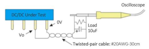
Diagram 2-3 Twisted-pair cable measuring method
