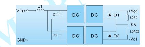
Diagram 3-5 Method 3 of DC/DC Converters connected in parallel
