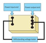
Diagram 2-7 Method of Withstand Test
