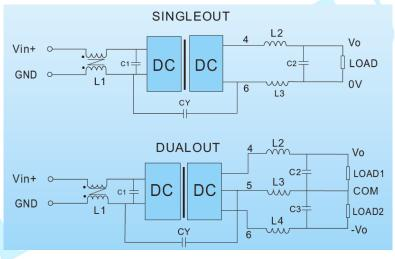
Diagram 3-72 Recommended circuit reducing ripple & noise
