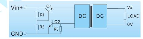
Diagram 3-10 Continuous over-current protection circuit
