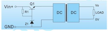
Diagram 3-9 Continuous over-voltage protection circuit
