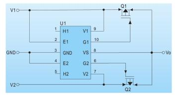
Diagram 3-4 Method 2 of DC/DC Converters connected in parallel
