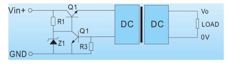
Diagram 3-61 Continuous over-voltage and over-current protection circuit
