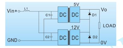
Diagram 3-1 Method 1 of DC/DC Converters connected in series
