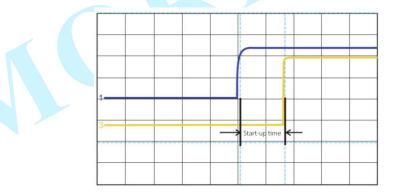
Diagram 2-6 Waveform of Start-up Time Test
