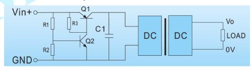
Diagram 3-7 Input under-voltage protection circuit
