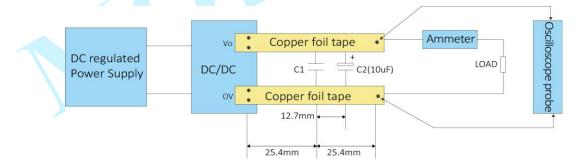
Diagram 2-2 Parallel cable measuring method
