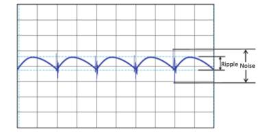
Diagram 2-5 Waveform of Ripple & Noise Test
