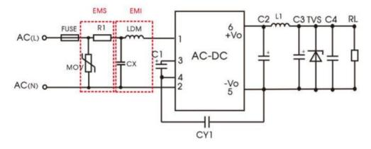
Figure 3-2 Typical application circuit of conventional LS series products (LO series products usually do not require peripheral circuits)
