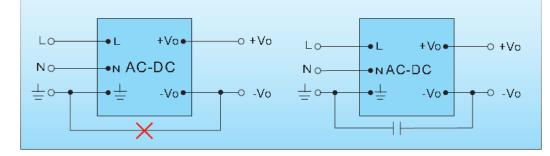
Figure 5-1 Connection of the output ground and the protective ground
