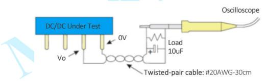
Diagram 4-2 Twisted-pair cable measuring method
