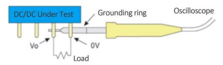
Diagram 4-3 Contact measuring method
