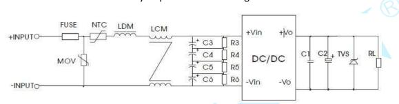
Diagram 3-1 EMC Solution-recommended Circuit
