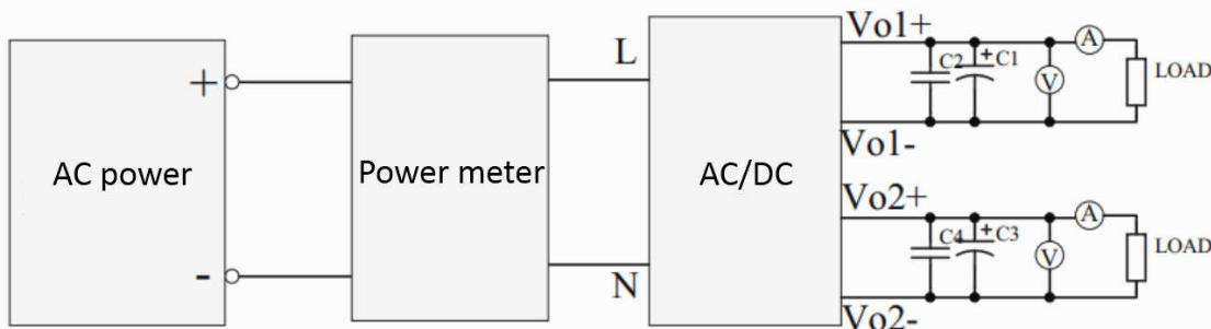
Figure 3-2 Multi-output basic test circuit connection
