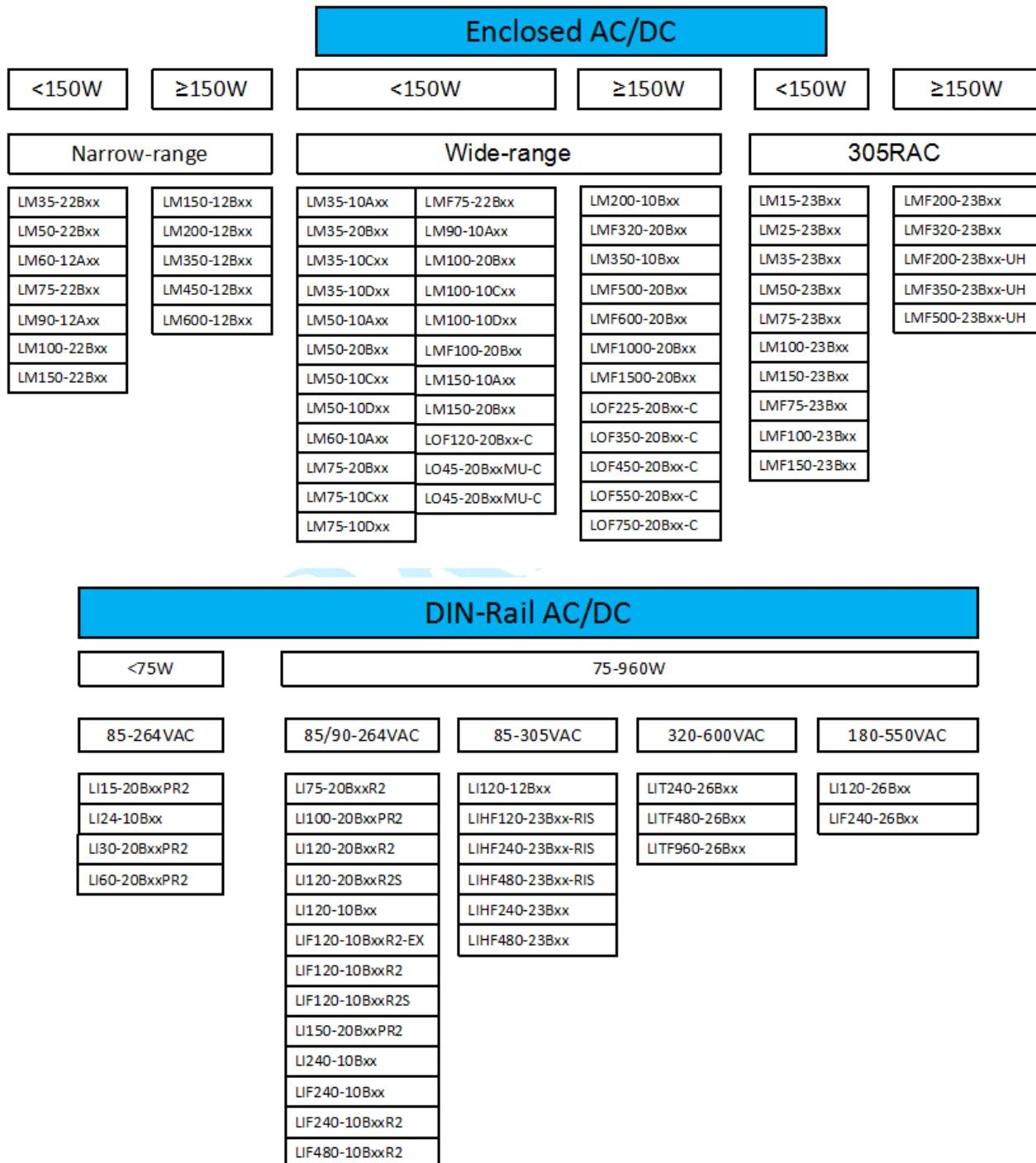
Figure 2-1 Enclosed/DIN-Rail AC/DC Selection Diagram
