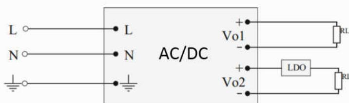
Figure 3-4 Typical application diagram of dual output
