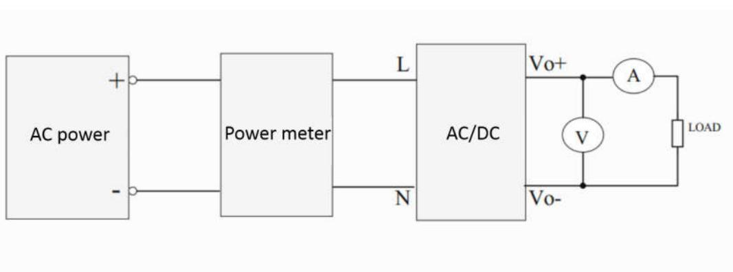
Figure 3-1 Single output product testing connection
