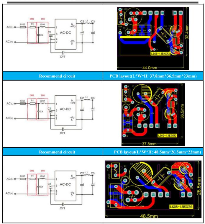
Note: There are three kinds PCB layouts are recommended for this solution. The first is for strict height requirement situations, and the second is for situations where length and width are required but the height is less limited. The third is for strict width requirement situations.
