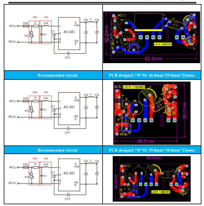
Note: Three PCB layouts are recommended for this solution. The first is to meet the occasions with strict requirements for height, the second is for occasions with requirements for product length and width, and the third is for occasions with strict requirements for width.
