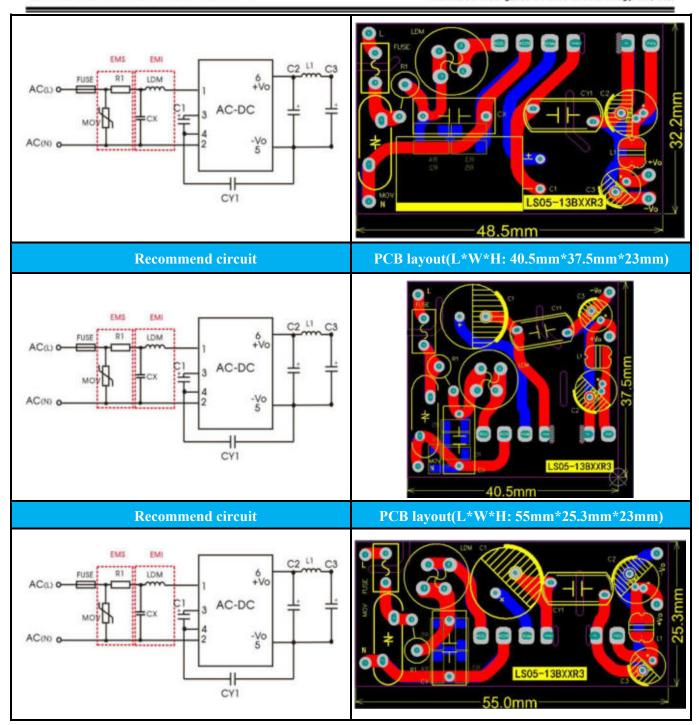
Note: There are three kinds PCB layouts are recommended for this solution. The first is for strict height requirement situations, and the second is for situations where length and width are required but the height is less limited. The third is for strict width requirement situations.
