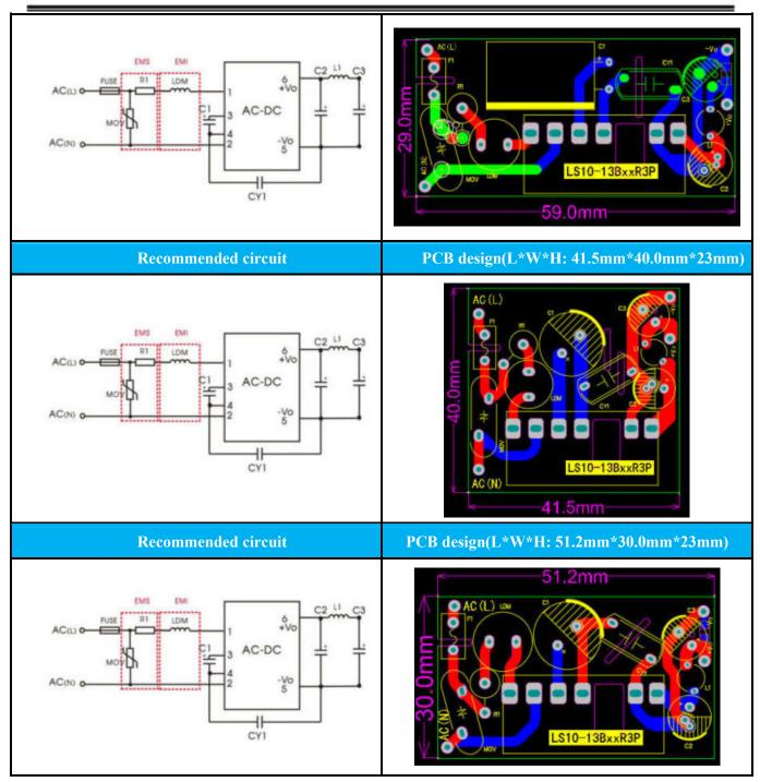
Note: Three PCB layouts are recommended for this solution. The first is to meet the occasions with strict requirements for Height, the second is for occasions with requirements for length, and the third is for occasions with strict requirements for wide.
