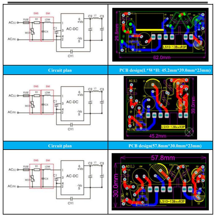
Note: Three PCB layouts were recommended to this solution. The first type is to meet the occasion that has requirement for height, the second one is for those has requirement for length and the last one is for those has requirement for Width.
