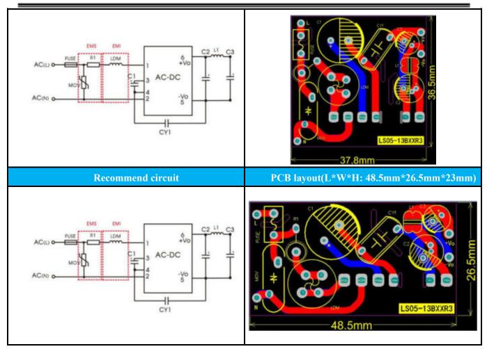
Note: There are three kinds PCB layouts are recommended for this solution. The first is for strict height requirement situations, and the second is for situations where length and width are required but the height is less limited. The third is strict for width requirement situations.
