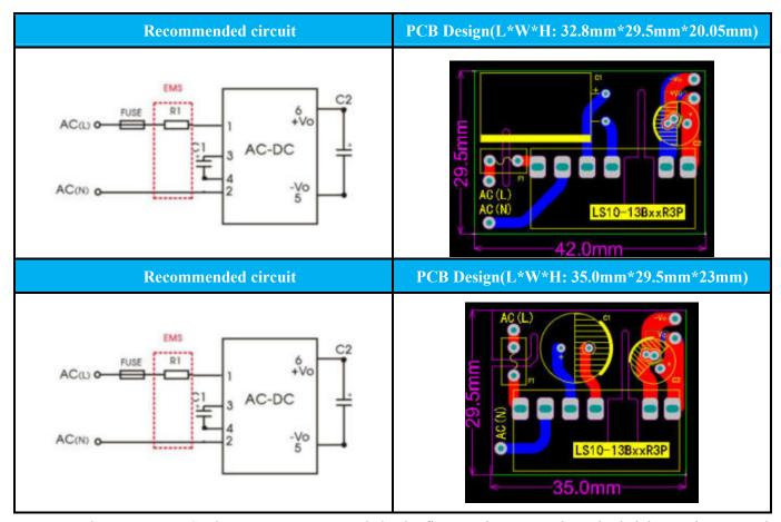
Note: There are two PCB layouts are recommended. The first one is to meet the strict height requirements, the second one is to meet the strict length and width requirements.
