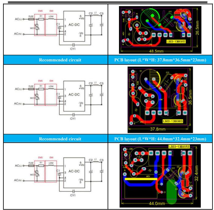
Note: There are three kinds of PCB layouts are recommended for this solution. The first is for strict height requirement situations, and the second is for situations where length and width are required but the height is less limited. The third is for strict width requirement situations.
