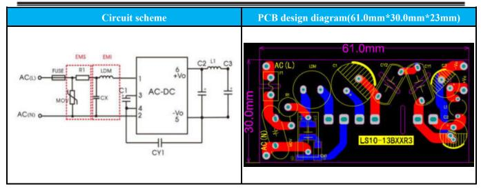
Note: Three PCB layouts are recommended for this solution. The first is to meet the occasions with strict requirements for height, the second is for occasions with requirements for product length and width, and the third is for occasions with strict requirements for width.
