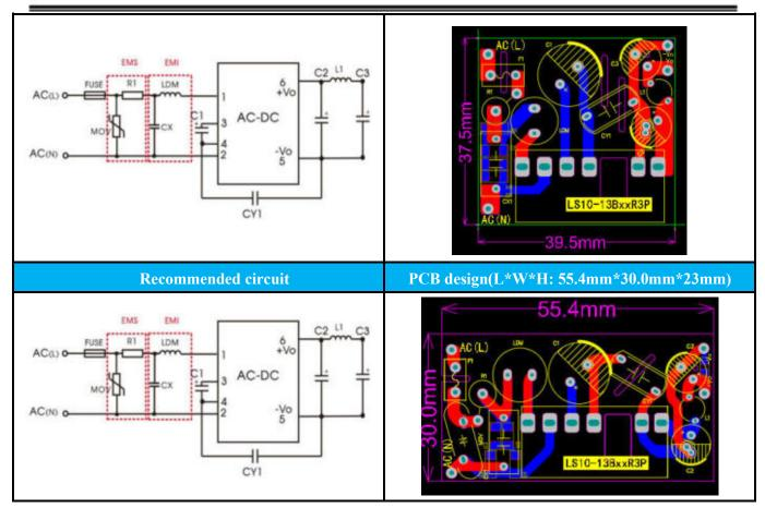
Note: Three PCB layouts are recommended for this solution. The first is to meet the occasions with strict requirements for Height, the second is for occasions with requirements for length, and the third is for occasions with strict requirements for wide.
