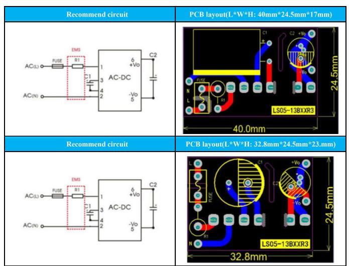
Note: There are two kinds PCB layouts are recommended for this solution. The first is for strict height requirement situations, and the second is for situations where length and width are required but the height is less limited.
