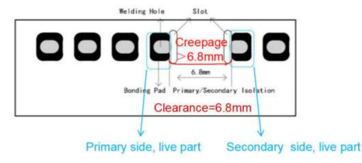
It can be seen from the figure that the electrical clearance refers to the shortest distance between the input terminal and the output terminal, and the creepage distance refers to the shortest distance from the primary terminal to the output terminal after bypassing the slotted hole.
