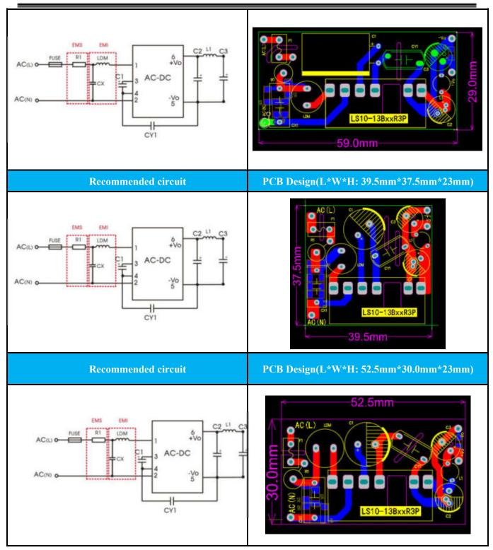
Note: There are three PCB layouts are recommended. The first one is to meet the strict height requirements, the second one is to meet the strict length and width requirements, and the third one is to meet the strict width requirements.
