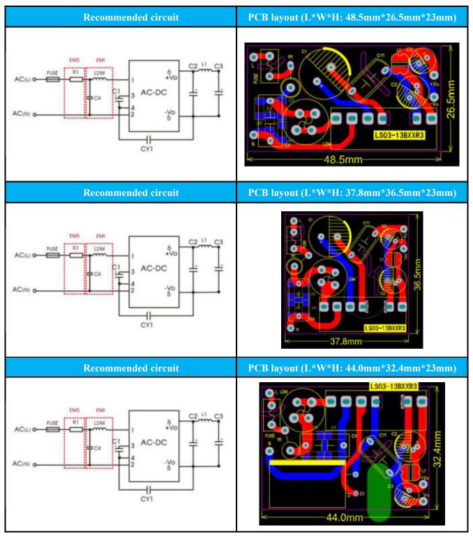
Note: There are three kinds of PCB layouts are recommended for this solution. The first is for strict height requirement situations, and the second is for situations where length and width are required but the height is less limited. The third is for strict width requirement situations.
