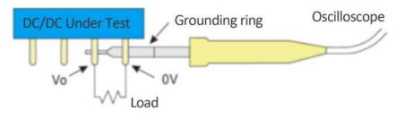
Diagram 4-3 Contact measuring method
