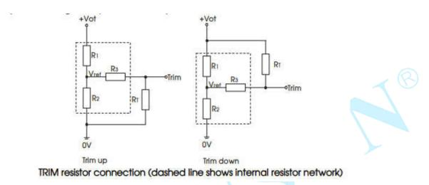
Diagram 4-6 Output Voltage Adjustment Schematic Diagram
