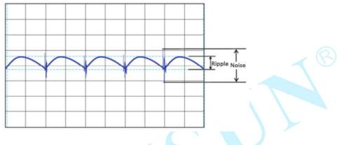
Diagram 4-4 Waveform of Ripple & Noise Test
