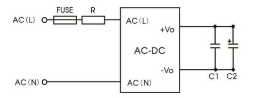
Diagram 3-1 EMC Solution-recommended Circuit
