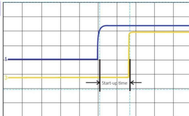
Diagram 2-7 Waveform of Start-up Time Test
