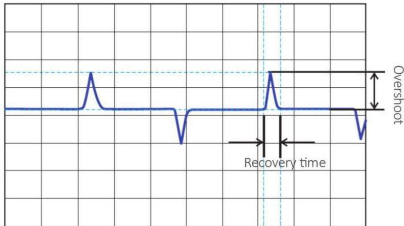
Diagram 2-6 Waveform of dynamic load Test
