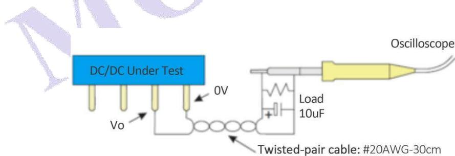
Diagram 2-3 Twisted-pair cable measuring method
