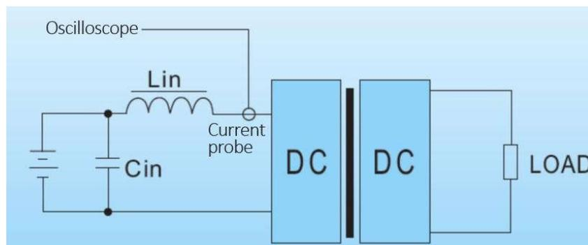
Diagram 2-11 Input Reflection Ripple Current Test
