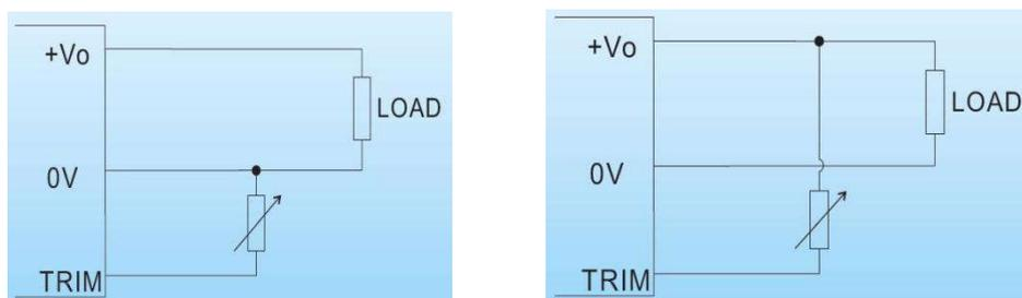
Diagram 3-3 Connection of output voltage's trimming with an external resistor
