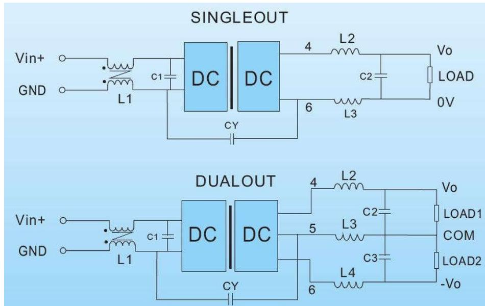
Diagram 3-1 Recommended circuit reducing ripple & noise
