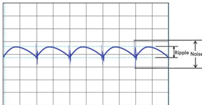
Diagram 2-5 Waveform of Ripple & Noise Test
