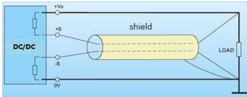
Diagram 3-4 Connection of remote control
