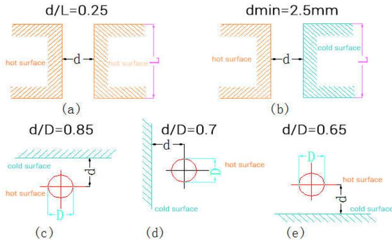
Diagram 1-2 the distance between the devices
