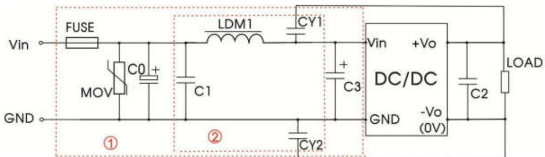
Diagram 3-2 EMC Solution-recommended Circuit
