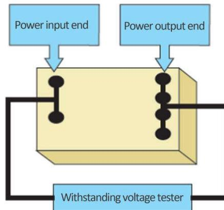
Diagram 2-8 Method of Withstand Test
