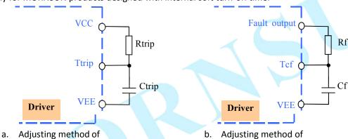
Diagram 17: Adjusting method of fault suppression time and soft turn-off time
