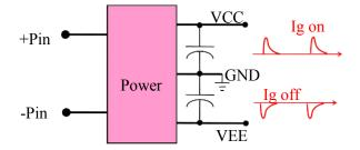
Diagram 14: Load condition of power supply for IGBT driver
