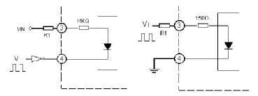
Diagram 8: Input method of IGBT driver
