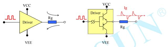
Diagram 12: Characteristics of IGBT driver output terminal
