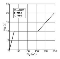
Diagram 13: Example of IGBT gate C/V changes
