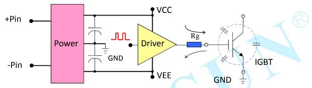
Diagram 3: Relations between IGBT, IGBT Driver and DC/DC converter for IGBT Driver
