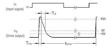
Diagram 16: Definitions of short-circuit detection time delay, soft turn-off time and protection reset time
