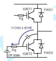
Diagram 21: Principle of wrongly triggering IGBT
