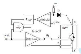
Diagram 15: Principle of fault detection and feedback
