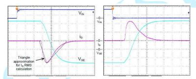
Diagram 11: Gate resistor current wave
