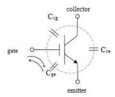
Diagram 1: Charging and Discharging Model of IGBT Gate
