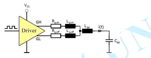
**Diagram 10: Typical IGBT Gate Drive Model**
