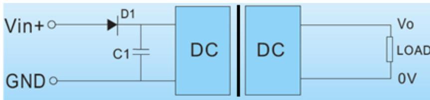
Diagram 3-6 Input reverse polarity protection circuit
