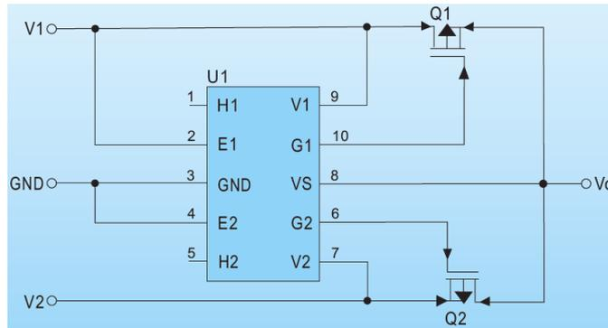
Diagram 3-4 Method 2 of DC/DC Converters connected in parallel
