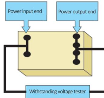
Diagram 2-7 Method of Withstand Test
