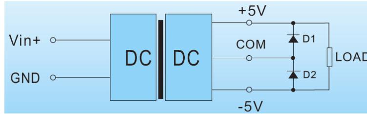
Diagram 3-2 Method 2 of DC/DC Converters connected in series
