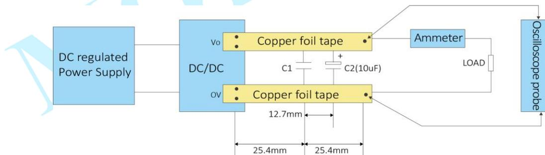
Diagram 2-2 Parallel cable measuring method
