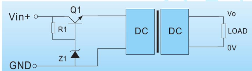
Diagram 3-9 Continuous over-voltage protection circuit
