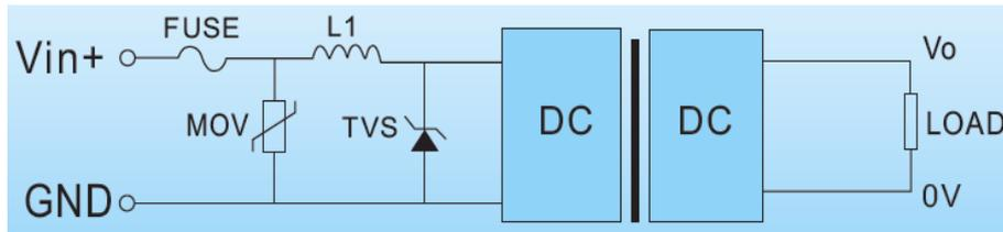
Diagram 3-8 instant over-current and over-voltage protection circuit
