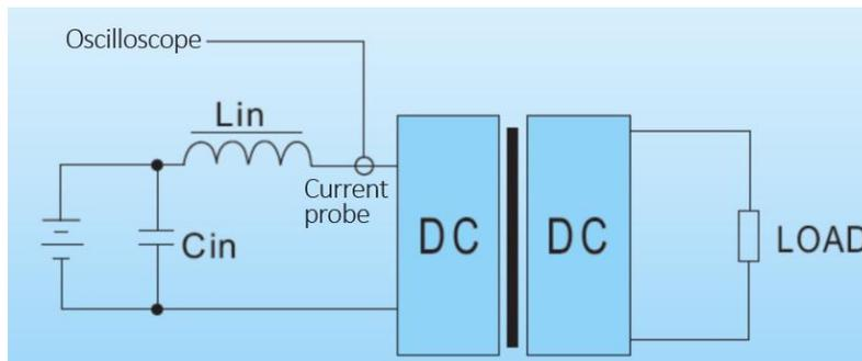
Diagram 2-9 Input Reflection Ripple Current Test
