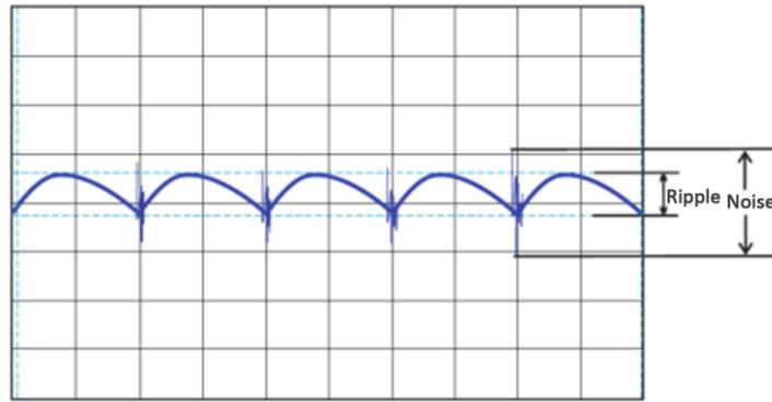
Diagram 2-5 Waveform of Ripple &amp; Noise Test
