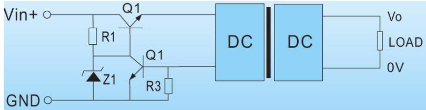
Diagram 3-61 Continuous over-voltage and over-current protection circuit
