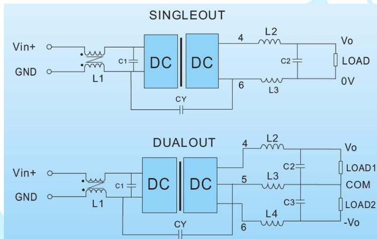
Diagram 3-72 Recommended circuit reducing ripple & noise
