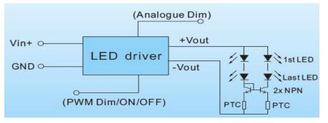
Diagram 3-2: LED Driver used in series and parallel
