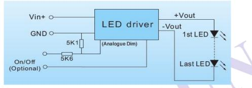
Diagram 3-3: Analog Dimming Application Circuit
