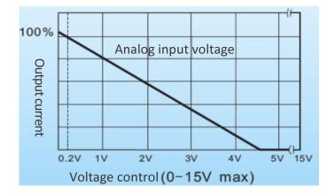
Diagram 3-4: Relationship of LED Driver between the regulation voltage and output current The spectrum and color temperature are changed with the brightness which is also a problem to use
