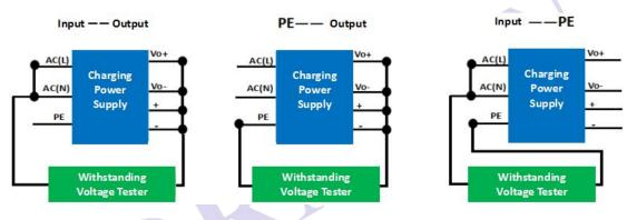
Figure 3-5: Withstand Voltage Test
