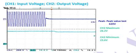
Figure 4-6: The Output UPS Voltage Waveform of Battery Charging Power Supply
