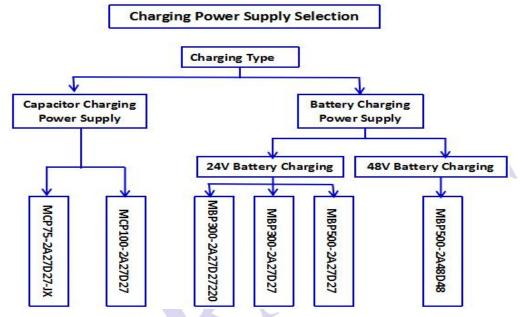
Figure 2-1: Selection Block Diagram
