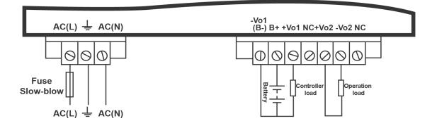
Figure 4-11: Pin Definition for 220VDC Output Charging Power Supply
