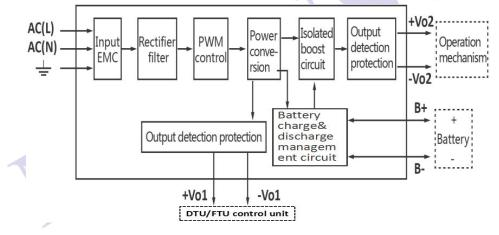
4.13 Typical Application Circuit for 220VDC Output Charging Power Supply
