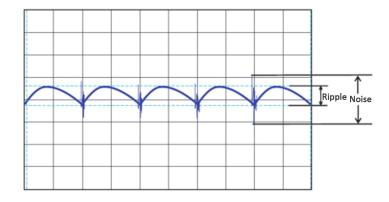
Figure 3-4: Ripple&Noise Test Waveform
