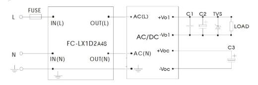
Figure 4-2: Typical Input EMC Filter Circuit
