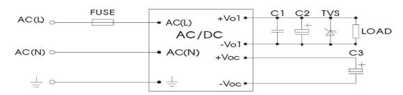
Figure 4-1: Typical Application Circuit of Capacitor Charging Power Supply
